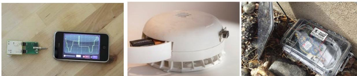
**Figure 1.** Three types of sensors (left to right): Add-on to cell phones (Project Hijack)<sup>53</sup>, Modified off-the-shelf (UCB-PATS)<sup>54</sup>, and purpose built standalone using existing circuit boards (solar-powered water sensor).<sup>55</sup>
